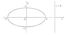
The area bounded by the ellipse  $x^2 + 4y^2 = 4$  is rotated about the line x = 3 to form an oblate torus.
